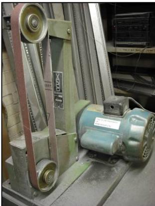
A **Vanco Flexiband model 1** bench 1" linisher serial no. 13748
