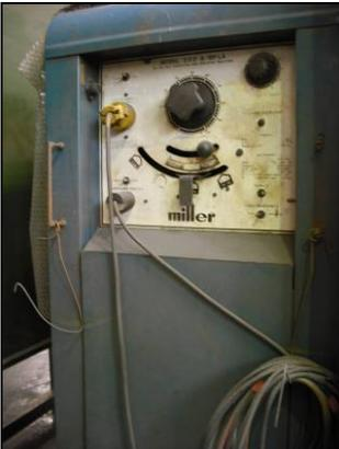
A **Miller model 320A/BP.LA AC/DC** gas tungsten arc welding machine(The Buyer of this lot will be required to provide a removal method statement for approval by the Seller or Agent prior to the removal of the lot)
