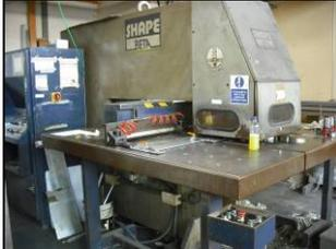
A **Shape Beta** punch press with DynaPath Systems Inc Delta 20 cnc control serial no. 35/220B complete with a quantity of tooling (The Buyer of this lot will be required to provide a removal method statement for approval by the Seller or Agent prior to the removal of the lot)
