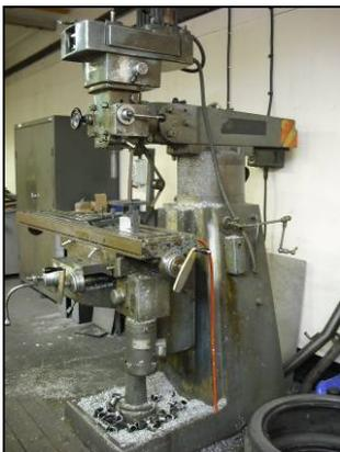
**A Balding Engineering Limited Beavermill VBRP adjustable speed turret milling machine with T slot powered bed, serial no. 10295\2** (The Buyer of this lot will be required to provide a removal method statement for approval by the Seller or Agent prior to the removal of the lot)
