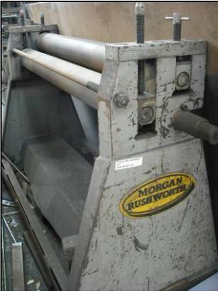
A **Morgan Rushworth** powered bending rolls approx. 50" width (The Buyer of this lot will be required to provide a removal method statement for approval by the Seller or Agent prior to the removal of the lot)
