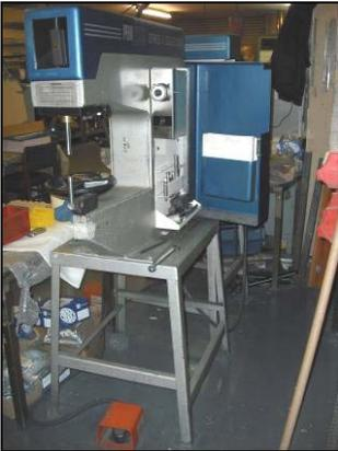
A **PEM Serter Series 4 6 ton** press no. J4 2331, on stand with 5.5 bar air supply, tool holder and foot switch(The Buyer of this lot will be required to provide a removal method statement for approval by the Seller or Agent prior to the removal of the lot)
