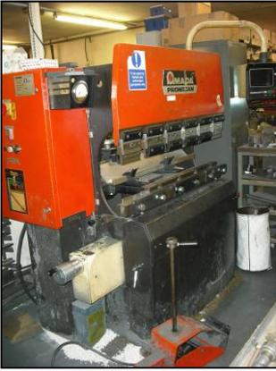
A 1988 **Amada Promecam IT2 25 ton** 1.2m hydraulic press brake no. IT2 025 12 4012 with Autobend 5C control, second axis, remote foot switch and a quantity of tooling (The Buyer of this lot will be required to provide a removal method statement for approval by the Seller or Agent prior to the removal of the lot)
