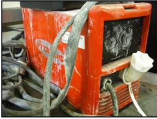
A **Fronius Magic Cleaner Stand Alone** weld cleaning machine no. 12041263
